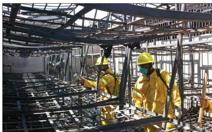
ATF investigators, pictured here, determined that the fire was accidental, the result of unintentional application of an open flame or smoking material to available combustibles, possibly to curtains surrounding the bunk beds. Photo: AP/Wide World.
